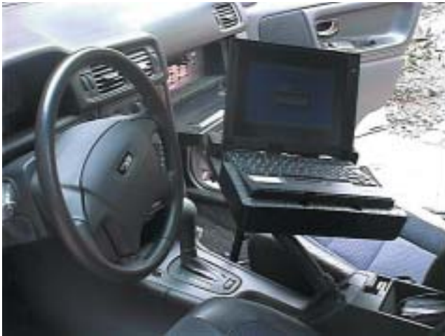
Figure 4: View of the Volvo Demonstrator Car showing the notebook connected to the ECU. The glove compartment (behind) contains the switchboard for controlling the built-in faults.
