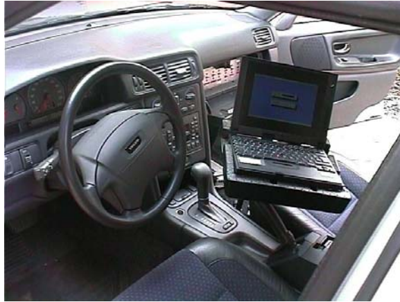
Figure 3: View of the Volvo 850 TDI Showing the Notebook Connected to the ECU. The Glove Compartment (Behind) Contains the Switchboard for Controlling the Built-in Faults.
